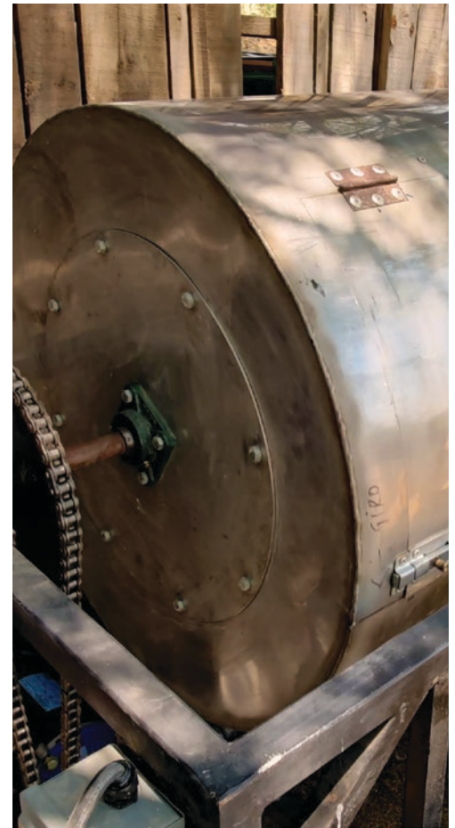
Propane rotational dryer with an electric motor, designed by Gerardo Ruiz Smith.
